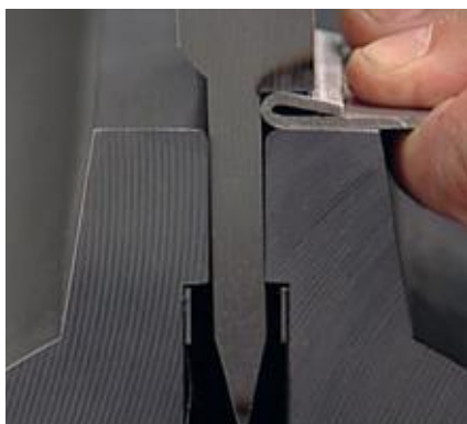
Pre-bend and flattening in the same tool.
