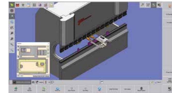
*EsaBend is an application for the programming and the simulation of a Press Brakes machines with a CNC, used to increase productivity, decrease downtime and reduce material wastage.*
